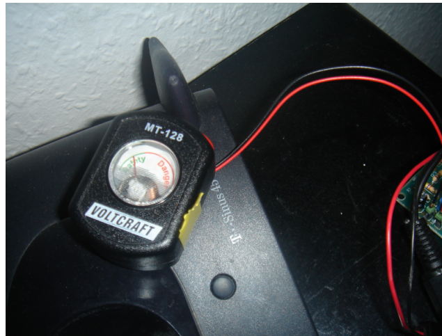
Figure 1: Arrangement for piezoelectrical pickup of field strength meter noises. The piezo is attached to the back of the meter.
